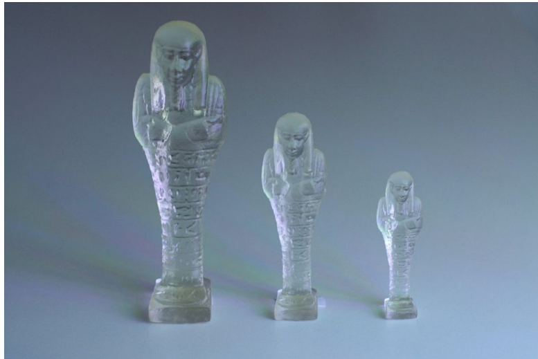
Fig. 4. 3D prints of the shabti figurine. Transparent clear resin prints at full and reduced sizes.
